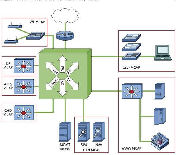
Figure 10 Zero Trust Network Architecture Is Segmented
